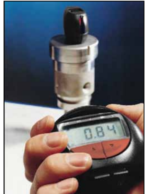
SR100 uses an infra-red (IrDA) link between the upper and lower units to provide remote, cable free operation up to a distance of 40" (one meter).
