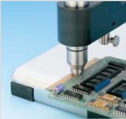
Typical measuring set-up: Measurement of gold layers on PCBs
