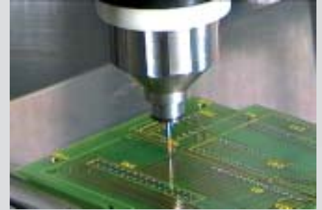
Centering unit for pinpoint cell positioning on small areas
